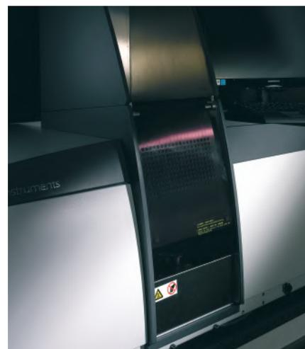
**AA500G** – The instrument is equipped with a Graphite Furnace Atomiser only. The graphite head is fixed into the optical path to maximise performance and eliminate drift.
