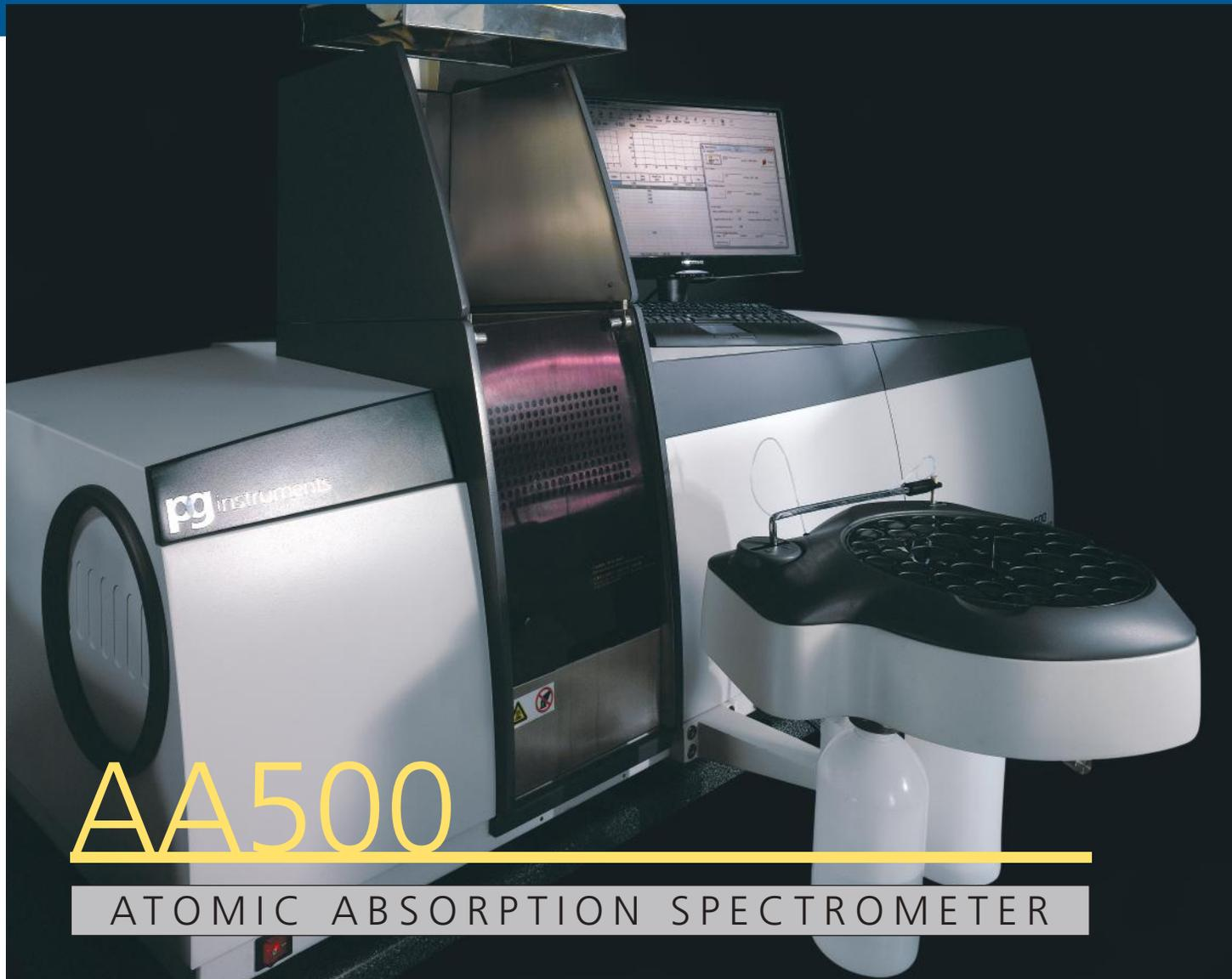
The AA500 Atomic Absorption Spectrometer is a high performance automated instrument designed to meet the requirements of the modern laboratory. Due to its versatility and performance it can be used for a wide range of applications including:
